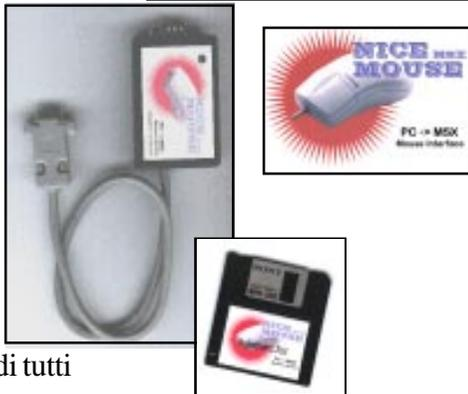
Nice Mouse is a little interface that it must to be connected at one of the joystick port and it permit at the users to using the PC mouse on own MSX computer.
