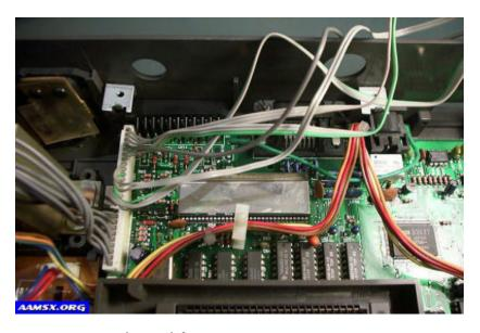
Now the board is (almost) free. It is still attached to the computer board by a flat cable plugged to it, but you don't need to unplug it. Just set the board aside so you can reach the disk drive cable, and unplug it.
