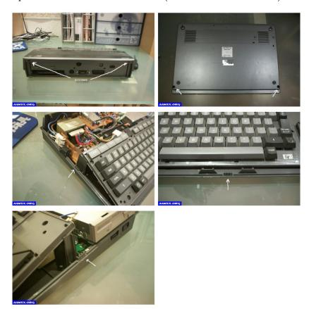
Be careful when you remove the cover, because there's a flat cable coming from the main board plugged to the LED board, as seen in the pictures. Just pull the plug to completely release the cover of the computer.
