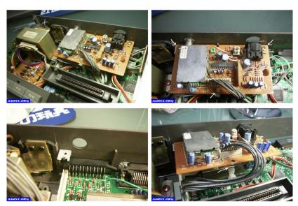
Be very careful when removing the screws on this board. They're screwed to small metallic pieces which are in turn screwed to the back plate of the computer. These metallic pieces are delicate, and could be damaged if you don't remove the screws carefully. Finally, remove the white plastic piece from its hole in the board. You might have to use pincers to push this piece while you pull it out from the hole.
