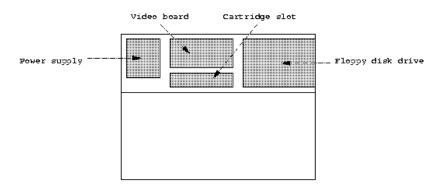
The disk drive is screwed to a metal plate, which is screwed to the computer board and has two small metal pieces inserted inside two small holes in the back cover. See the pictures for more detail. First remove the screws, and then carefully remove the drive and metal plate. Now carefully remove the two flat cables wired to the drive. The one with four wires is the drive's power supply.
